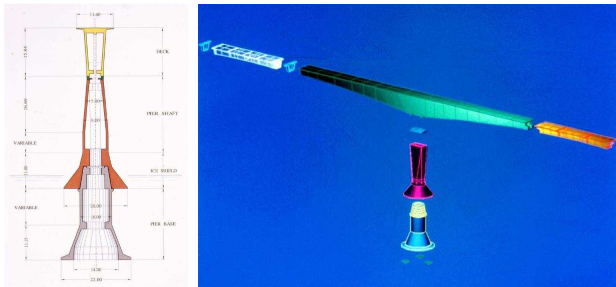
Figure 3 : Confederation Main Bridge – Concept and Prefabricated units
